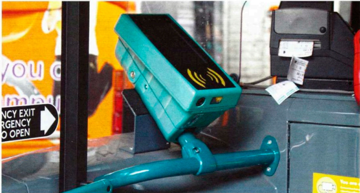
One of the INIT ITS0-compliant card readers which NCT is using
