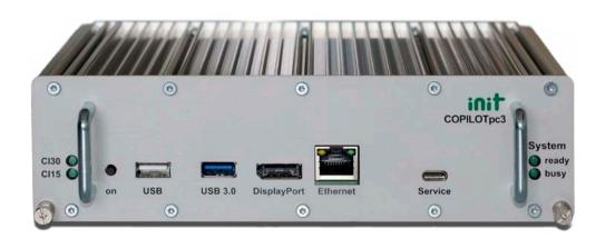
Today's ITS applications impose particularly high requirements on the performance of on-board computers and call for the exchange of large volumes of data between vehicle and control center. INIT responds to this challenge with COPILOTpc3. With a more powerful processor and its extended storage capacity, this vehicle IT and communication platform sets new standards in terms of performance.
