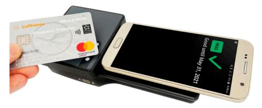
PROXreader2 can be used with an Android smartphone as an all-in-one ticket handling solution.
